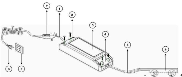
Screw the protection covers of input side and outside. Then connect the input cable and output cable on the connectors according to the drawing of input side and output side. Two 3mm screw holes on the bottom of housing can be used for fixing the device. When all is done put the protection covers back and screw fixed.
